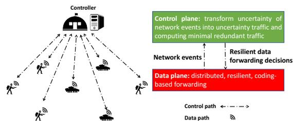
Fig. 1. The architecture of resilient, coding-based SD-MTN.
