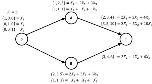
Fig. 2. An illustration of NC-based routing. The destination can decode a batch of  $K$  original packets as long as it receives  $K$  linearly independent coded packets.
