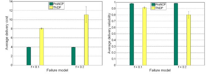
(a) Delivery cost under different node failure models. (b) Reliability under different node failure models.
