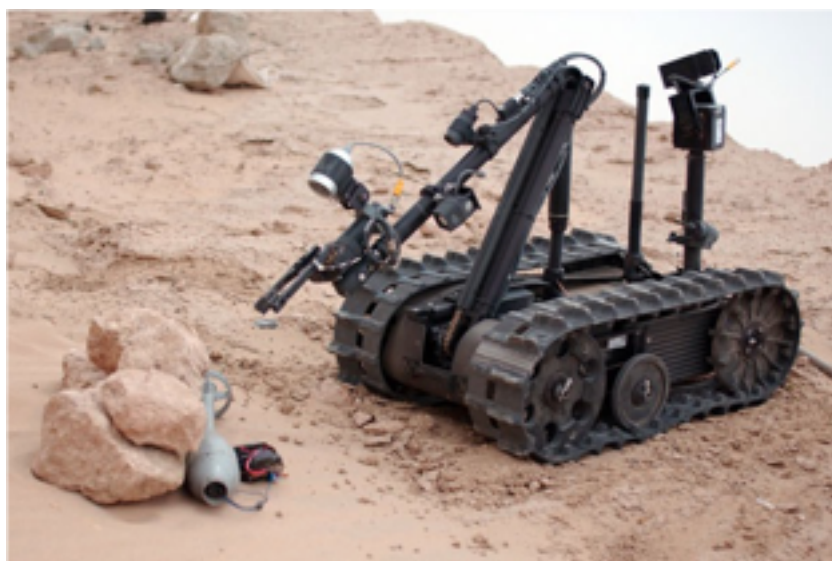
Figure 3: TALON Tracked Military Robot locates potential ordnance.
